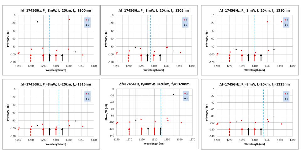
Interleaving polarization between CWDM channels effectively pushes any phase matched tones out of the US CWDM band. However PMD in the transmission fiber prevents maintaining the orthogonal polarizations. While not completely effective, it will reduce the FWM impairment somewhat since channels are partially orthogonal for first few kilometers.
