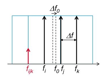
Peak FWM power increases for longer fiber spans and higher launch power, independent of grid.
