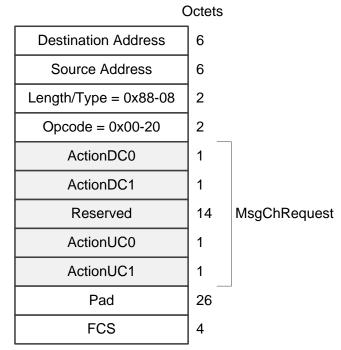
Figure 144-27 – Format of CC\_REQUEST CCPDU
