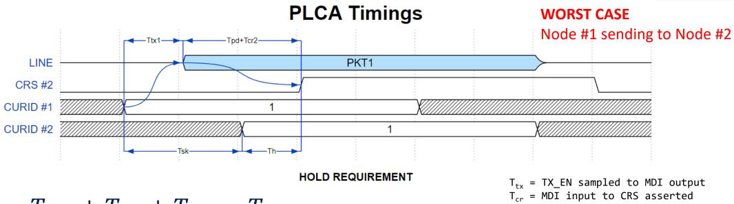
$$T_h = T_{tx1} + T_{pd} + T_{cr2} - T_{sk}$$
