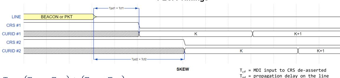
$$T_{sk} = (T_{pd2} - T_{pd1}) + (T_{cf2} - T_{cf1})$$
