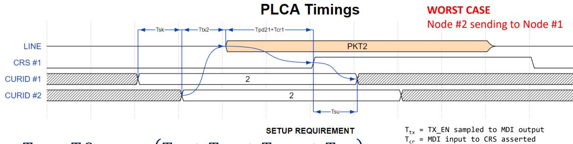
$$T_{su} = TO_{timer} - (T_{sk} + T_{tx2} + T_{pd12} + T_{cr1})$$
