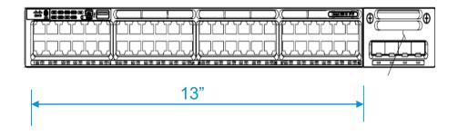
Future 96 port Switch (1RU) using Single Pair Stacked connectors 22 AWG to 26 AWG
