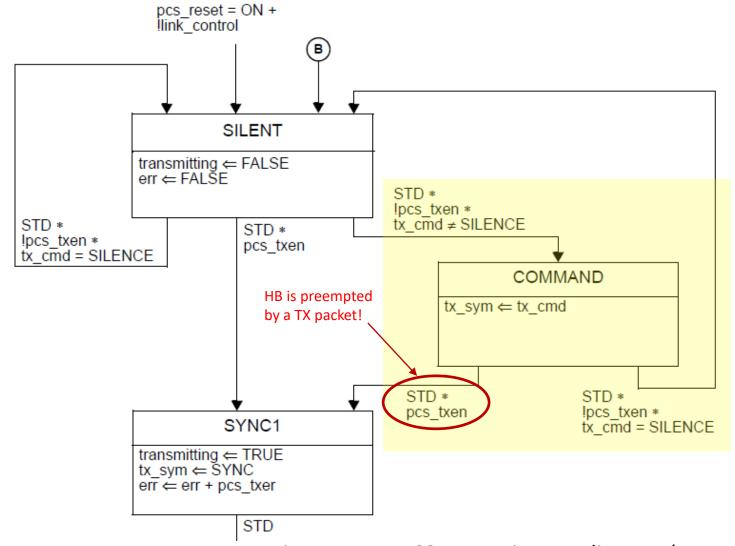
Figure 147-4 PCS Transmit state diagram (part a)
