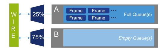
Observation: Node A is limited to 25% link capacity, but node B has no data → 75% link capacity is wasted
