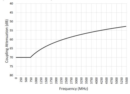
Figure 149–44—Coupling attenuation calculated using Equation (149–24)
