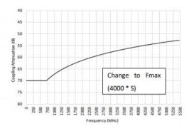
Figure 149-31: Coupling attenuation calculated using equation (149-26)
