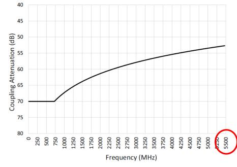
Figure 149–44—Coupling attenuation calculated using Equation (149–24)
