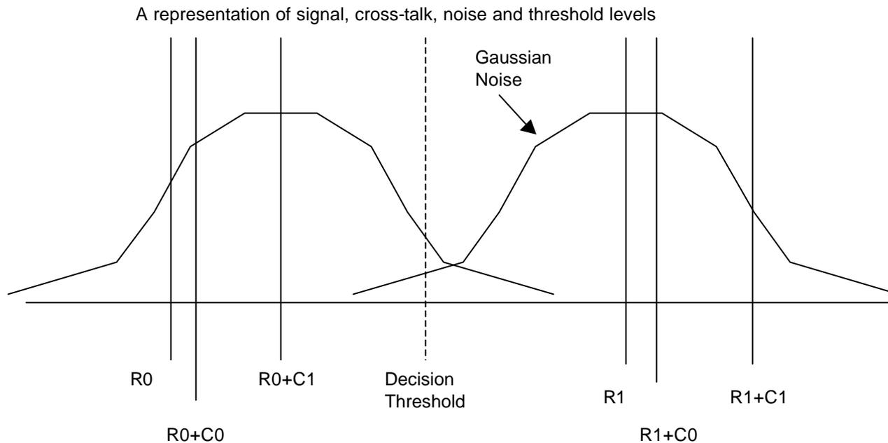
$R_0$  and  $R_1$  are receive power levels of transmitted signal binary 0 and 1, respectively.  $C_0$  and  $C_1$  are receive power levels of reflected signal binary 0 and 1, respectively.
