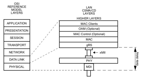
Figure 90–3—Data delay measurement
