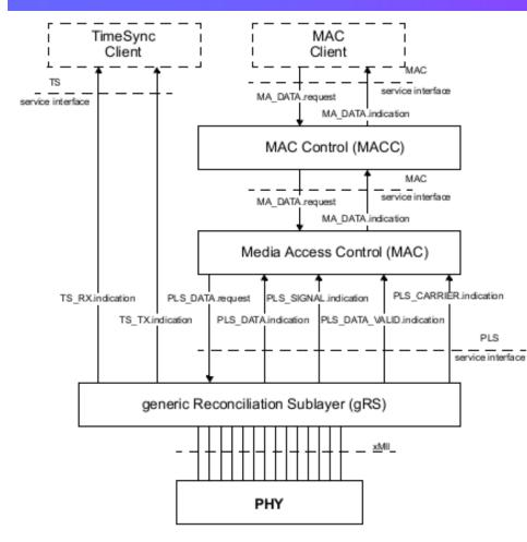
Shows source / destination for TS\_RX and TS\_TX indication primitives
