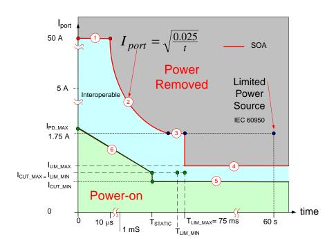
Real PD DC-DC operate near 100 kHz (T =  $10\mu$ s). What are our needs for real repetitive current ripple?
