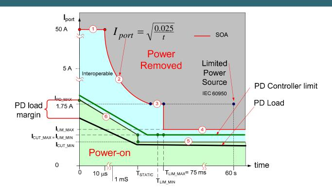
The PD design ensures the average current is within the green zone and may draw the maximum allowable power.
