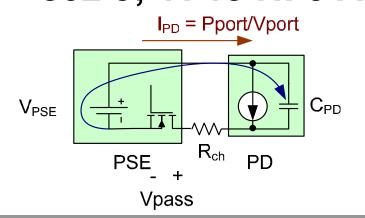
Worst-case Rch = 0 Vpse goes from 50 to 57 V Vpass goes from 0 to 7 V I<sub>PD</sub> = 400/350 x Pport/Vport
