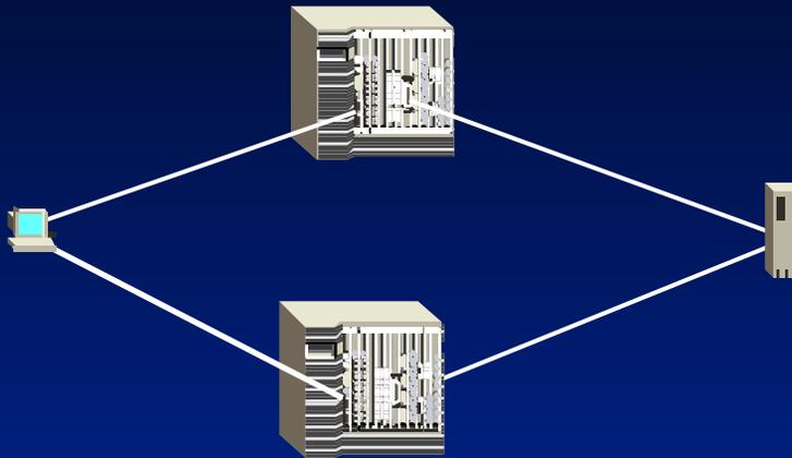
Both desktop and server see two links trunked together, but these links are supported by different switches to provide network redundancy
