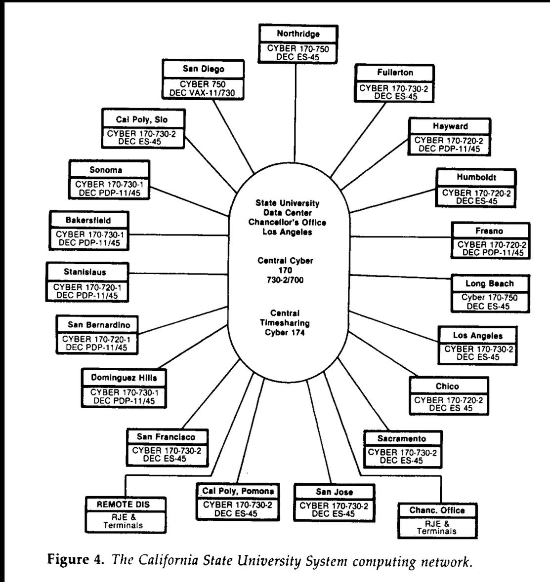
Figure 4. The California State University System computing network.
