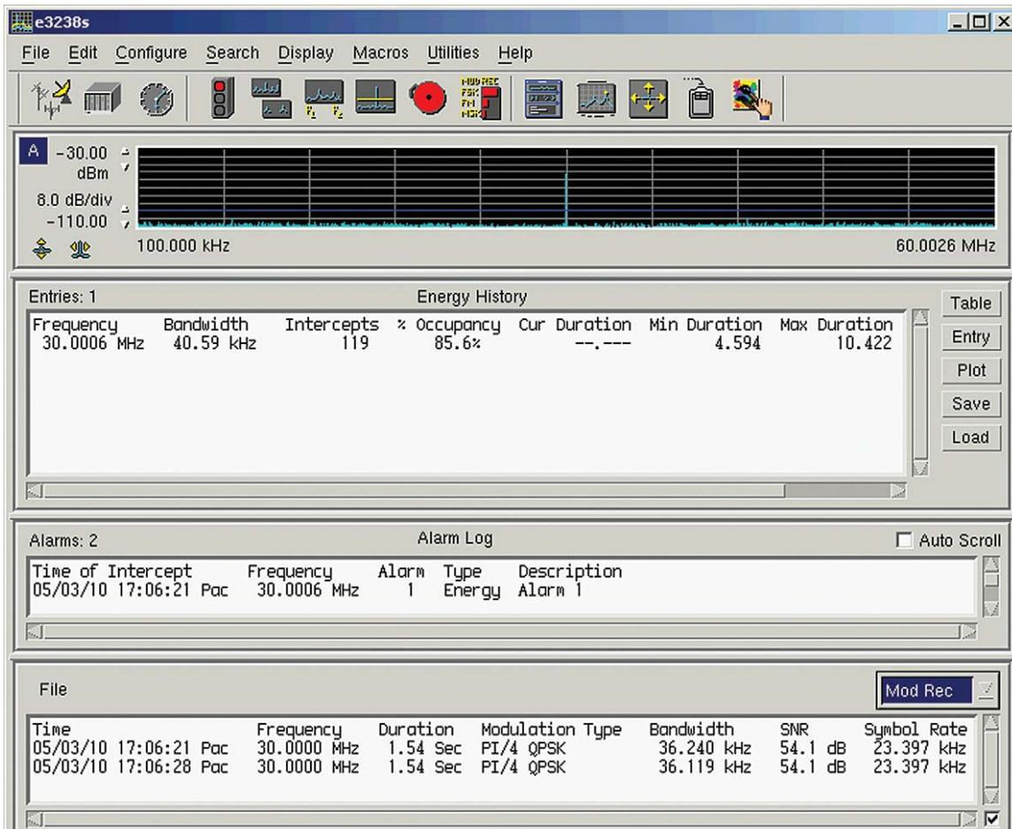
Figure 2: Screen Capture from E3238S GUI
