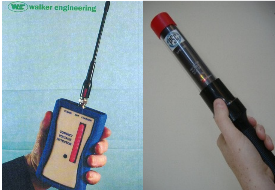
Figure 19 Examples of handheld electric field detectors which can be used to check ground references for voltage (Power Survey Co EFD-100 and Walker Engineering Contact Voltage Detector pictured)
