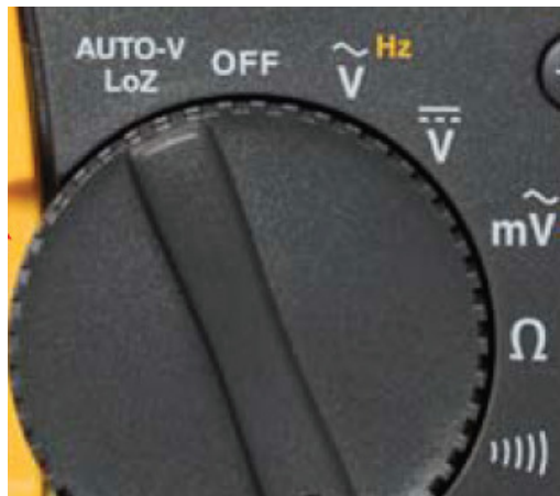
Figure 17 Digital Voltmeter with low impedance voltage measurement option built in (Fluke Model 117 shown as representative example)
