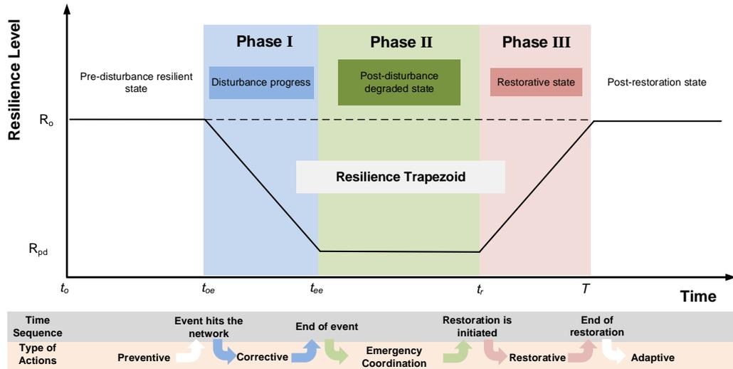
Fig. 1: The resilience trapezoid associated with an event (courtesy of M. Panteli)
