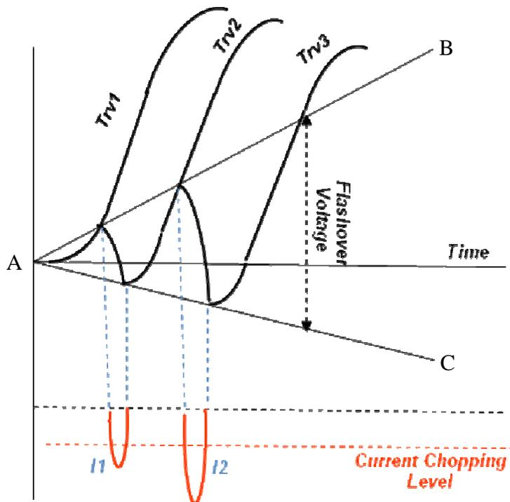
Fig. 1C. Transient produced by breaker re-ignitions.
