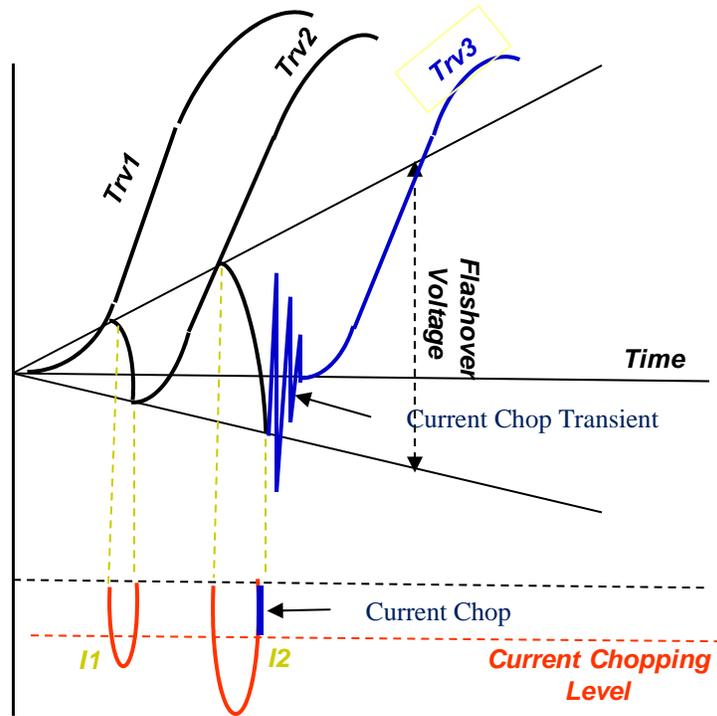
Fig. 1D. Re-ignition transient caused by current chopping.
