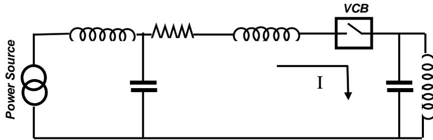
Fig. 1B. Lumped parameter equivalent circuit of the circuit shown in Fig. 4A
