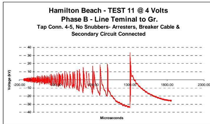
Fig.2 Recorded re-ignition transient at substation.
