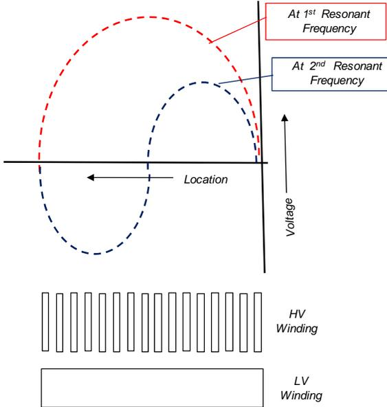
Fig. 4 Spacial voltage distribution at first and second resonant frequencies.
