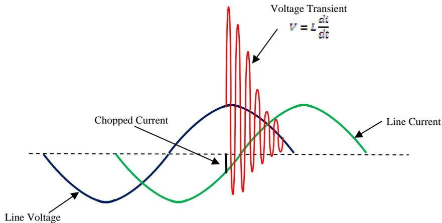
Fig. 1E Current chopping transient without re-ignitions
