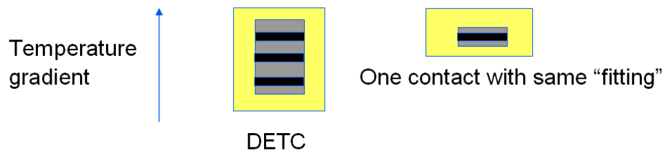
Fig. 8. Placement of contacts in test tank and temperature gradient influence
