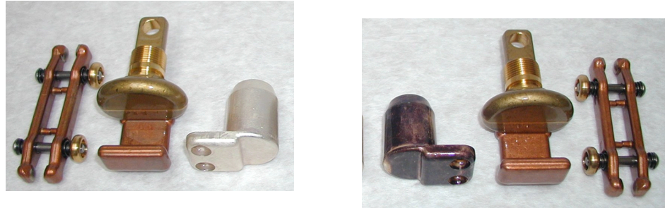
Fig. 7. Contacts stored in above oils for 22 days at 105°C
