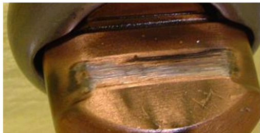
Fig. 3. Copper contact after several maneuvers against a silver contact.
