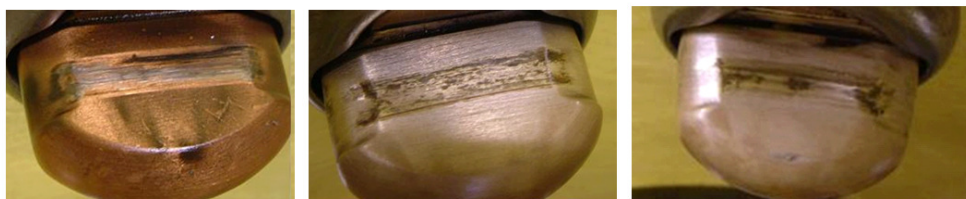
Fig. 9. Wiping effect on contacts
