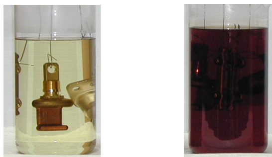
Fig. 6. Changes in oil appearance for 2 different oils after 22 days at 105°C
