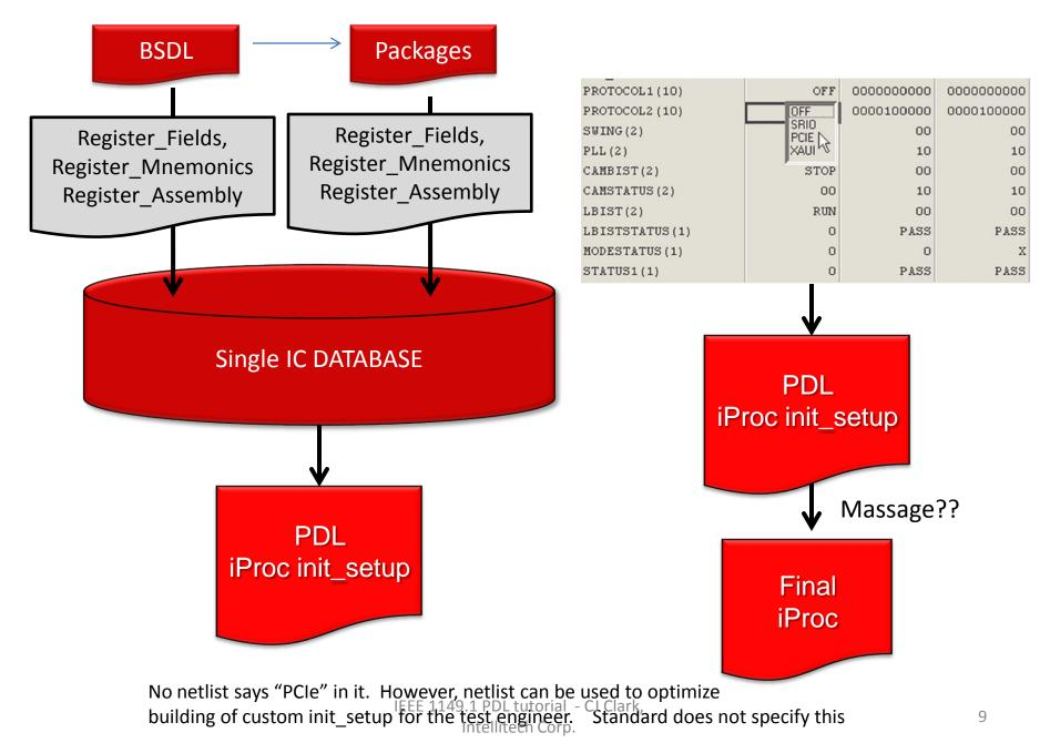
IP provided init\_setup for IO. Parameters passed in - not practical for 1000 I/O with four parameters each
