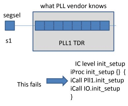
Like board level Scan Path Linkers, tool is responsible for opening SEGSELs, turning on DOMCTRL
