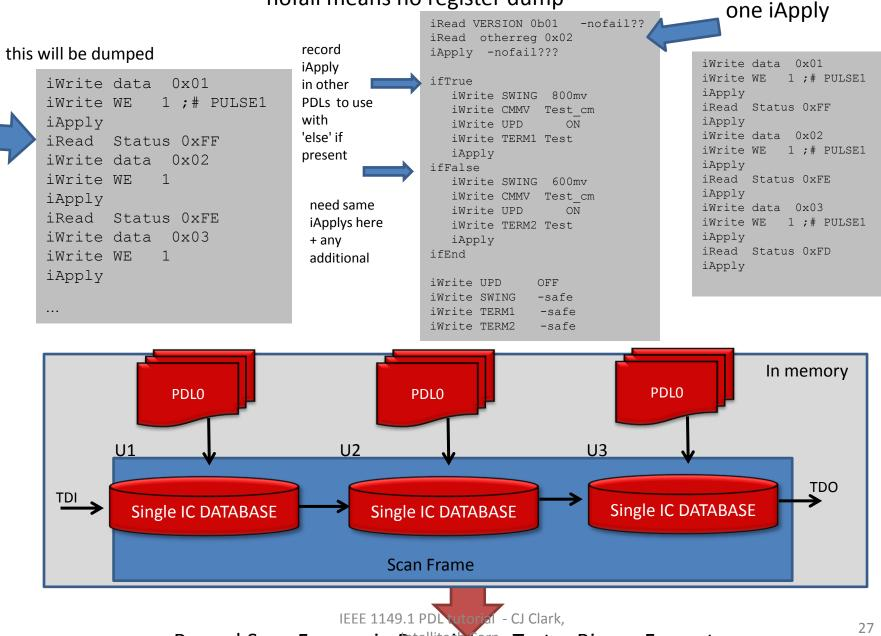
Record Scan Frames in Proprietary Tester Binary Format
