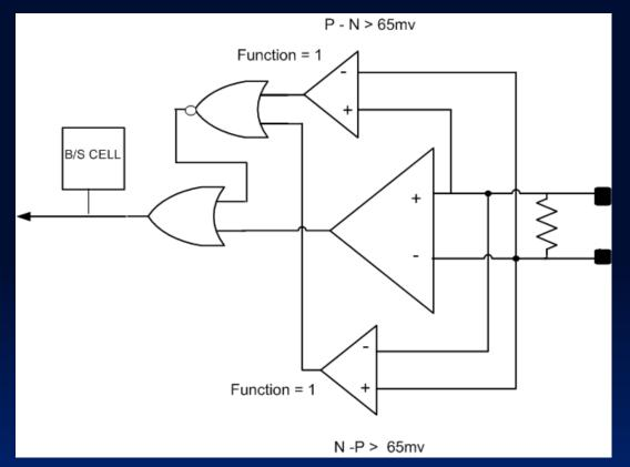
LVDS requires open inputs to cause differential receiver to drive '1'
