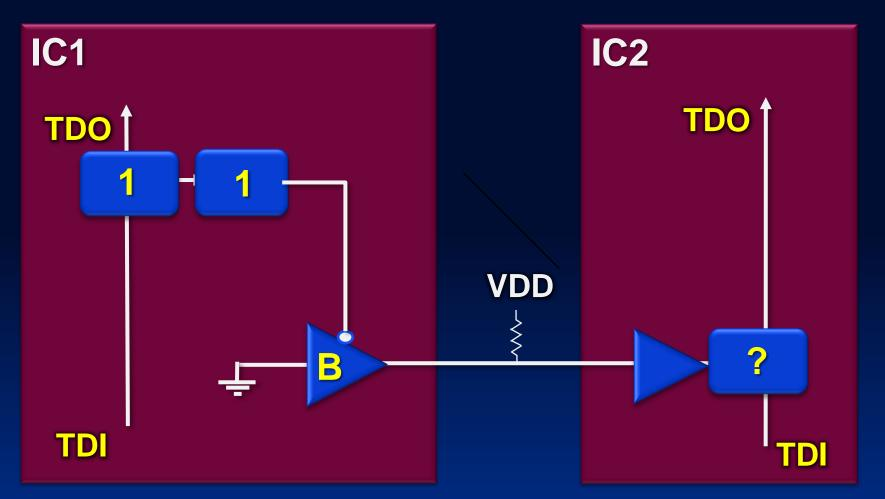
ATPG predicts a Logic 1 – well known Voltage at VDD or resistance precise resistance value not needed
