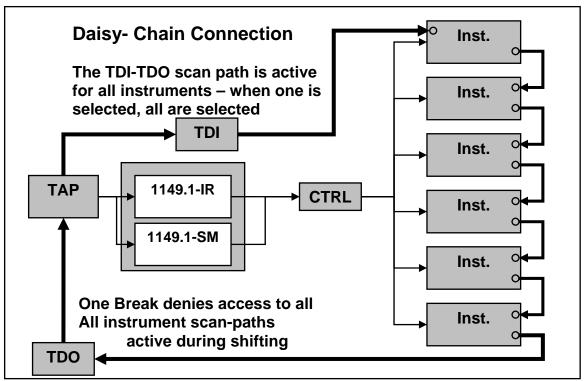
Figure 10: Example Daisy-Chain-Connection
