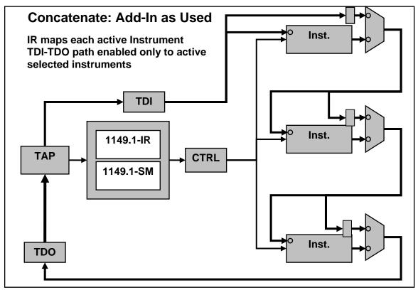
Figure 12: An example Concatenate-Connection
