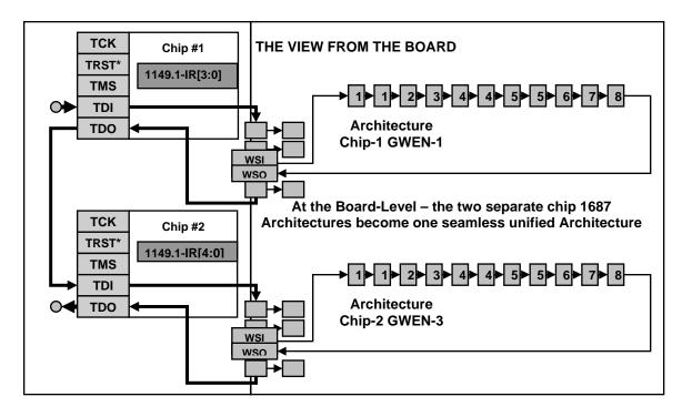
Figure 6: Example of Two 1687 Devices Concatenated on a Board
