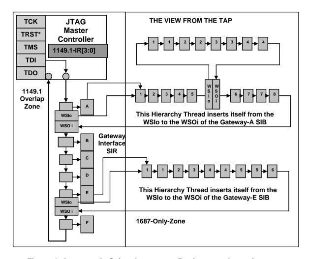
Figure 4: An example Select-Instrument-Register used as a Gateway
