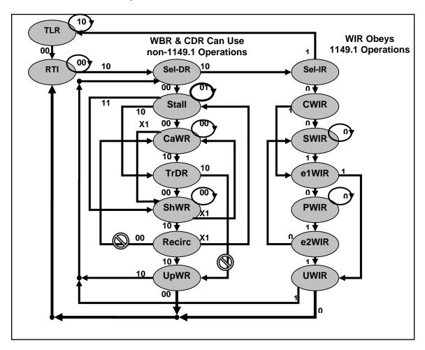
Figure B-2: An example Complex 1500-TAM+Transfer State-Machine
