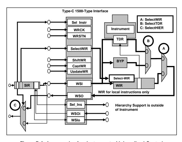
Figure B-6: An example of an Instrument with Localized-Control
