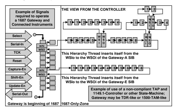
Figure 5: An example of the 1687 starting at the Gateway
