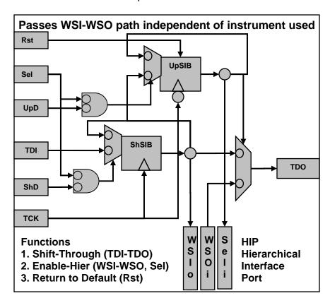
Figure 2: The Select-Instrument-Bit Concept as a Gateway Bit
