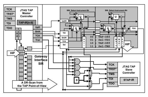
Figure B-3: An Example State-Machine Instrument Conversion
