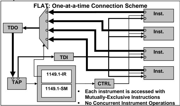
Figure 9: Example Flat-Connection
