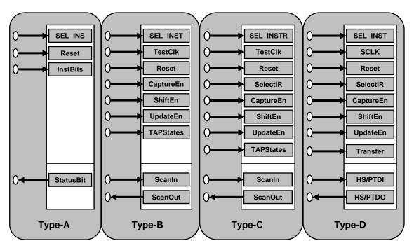
Figure 7: Example ABCD-Taxonomy Instrument Interfaces
