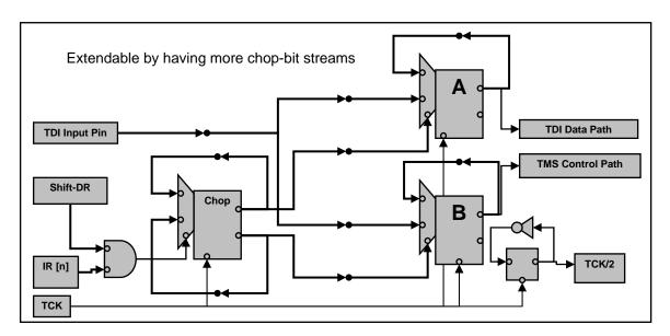
Figure B-4: An example Sequential TDI-Data Chopper
