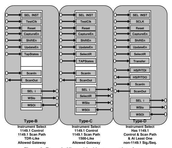
Figure 8: Example Hierarchical Instrument Interfaces
