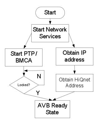
The device upon boot-up will start up PTP service. In parallel the device will obtain an IP and HiQnet address as per normal device behavior.
