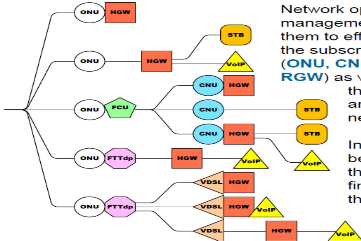
Network operators require a management system that would allow them to efficiently access and manage the subscriber demarcation device (**ONU, CNU, CM, DSL modem, or RGW**) as well as the various devices that interconnect their optical and copper sections of the network (**DPU or FCU**).
