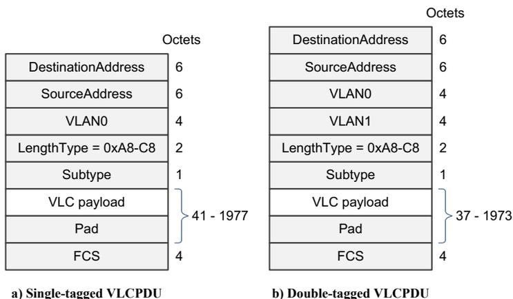
13 a) Single-tagged VLCPDU                      b) Double-tagged VLCPDU
