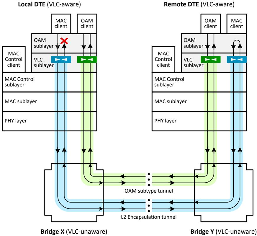
Figure 7-3—Remote OAM loopback over VLC tunnel with VLC-aware local DTE and VLC-aware remote DTE.
