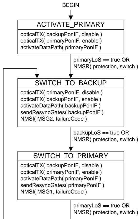
Figure 9-5—Trunk protection process operating on the OLT
