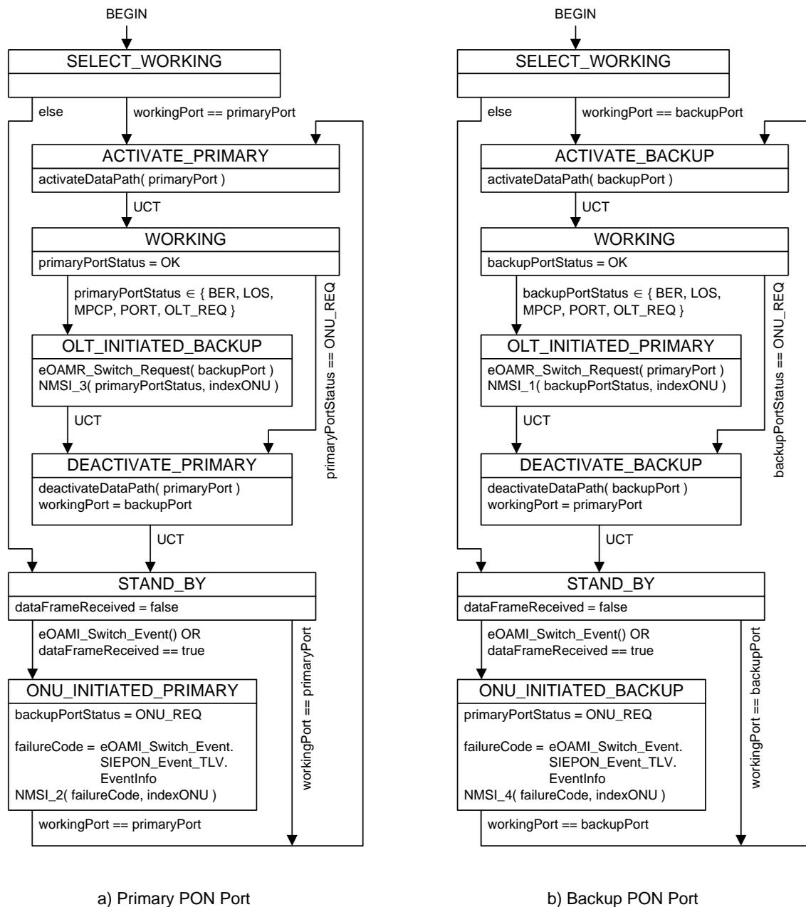
Figure 9-13—Tree protection process operating on the OLT
