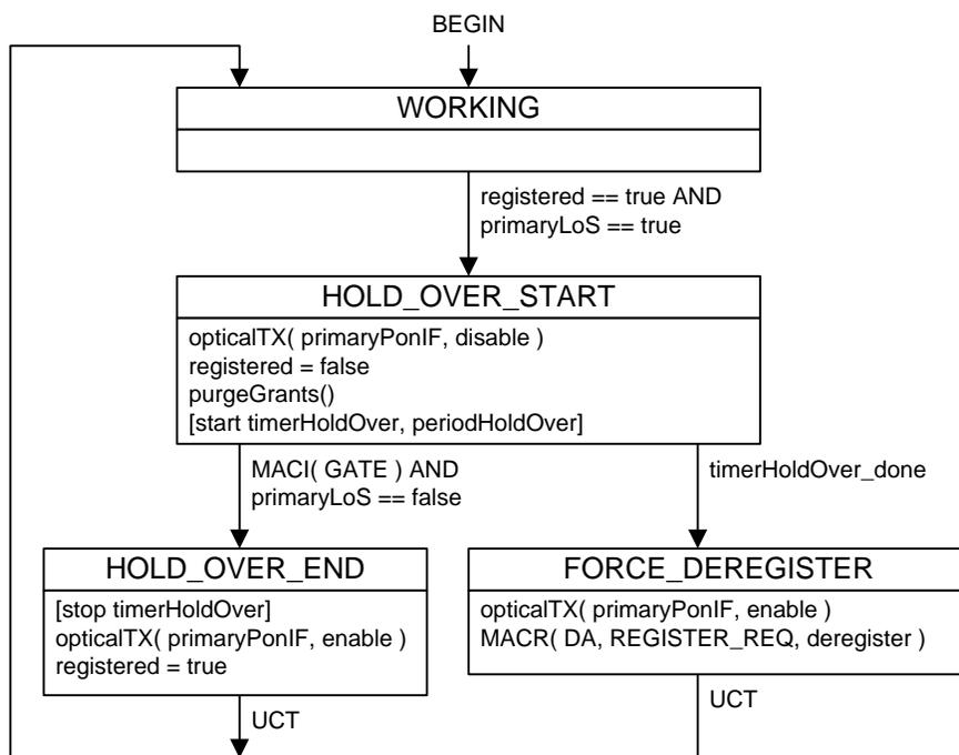
Figure 9-6—Trunk protection process operating on the ONU
