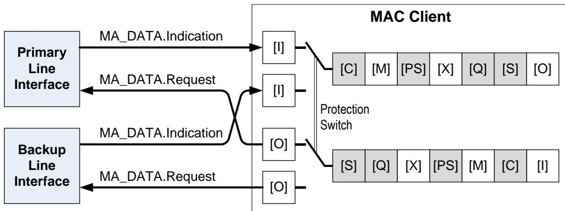
Figure 9-1—Line device protection architecture
