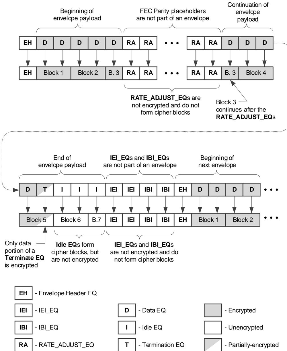
Figure 11-xx6 – Handling of special EQ types by encryption/decryption function
