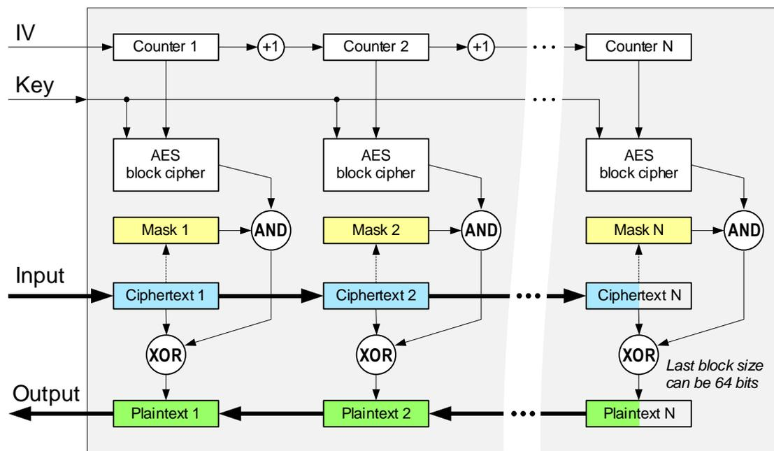
Figure 11-xx2 – Block diagram of the decryption process
