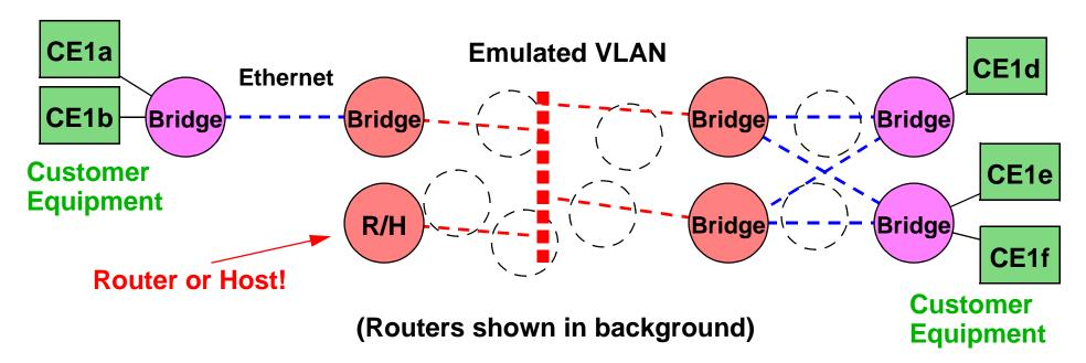
PE-rs becomes a bridge plus an Emulated VLAN. and bridge functions. Multi-Tenant Unit Switch (MTU-s) is a bridge, and may be Provider or Customer owned.
