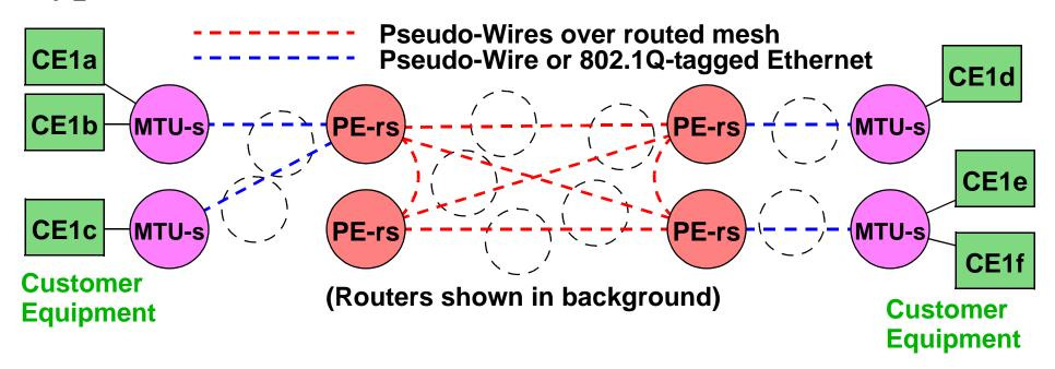
Lack of redundancy prevents loops
