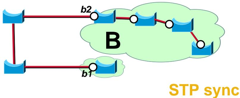
Domain B is split, *b1* and *b2* are root forwarding. A link is then brought up between the two parts.
