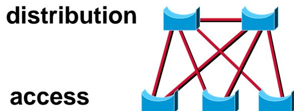
**If the uplinks of the access bridges are configured as L2GPs, the access will never provide redundancy for the distribution.**
