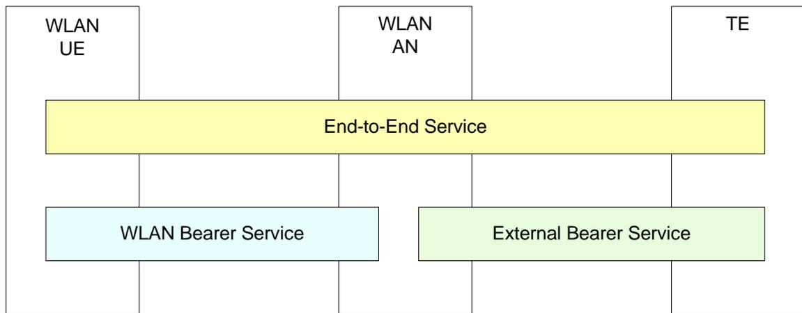
Figure 5.1 QoS Architecture for WLAN Direct IP Access
