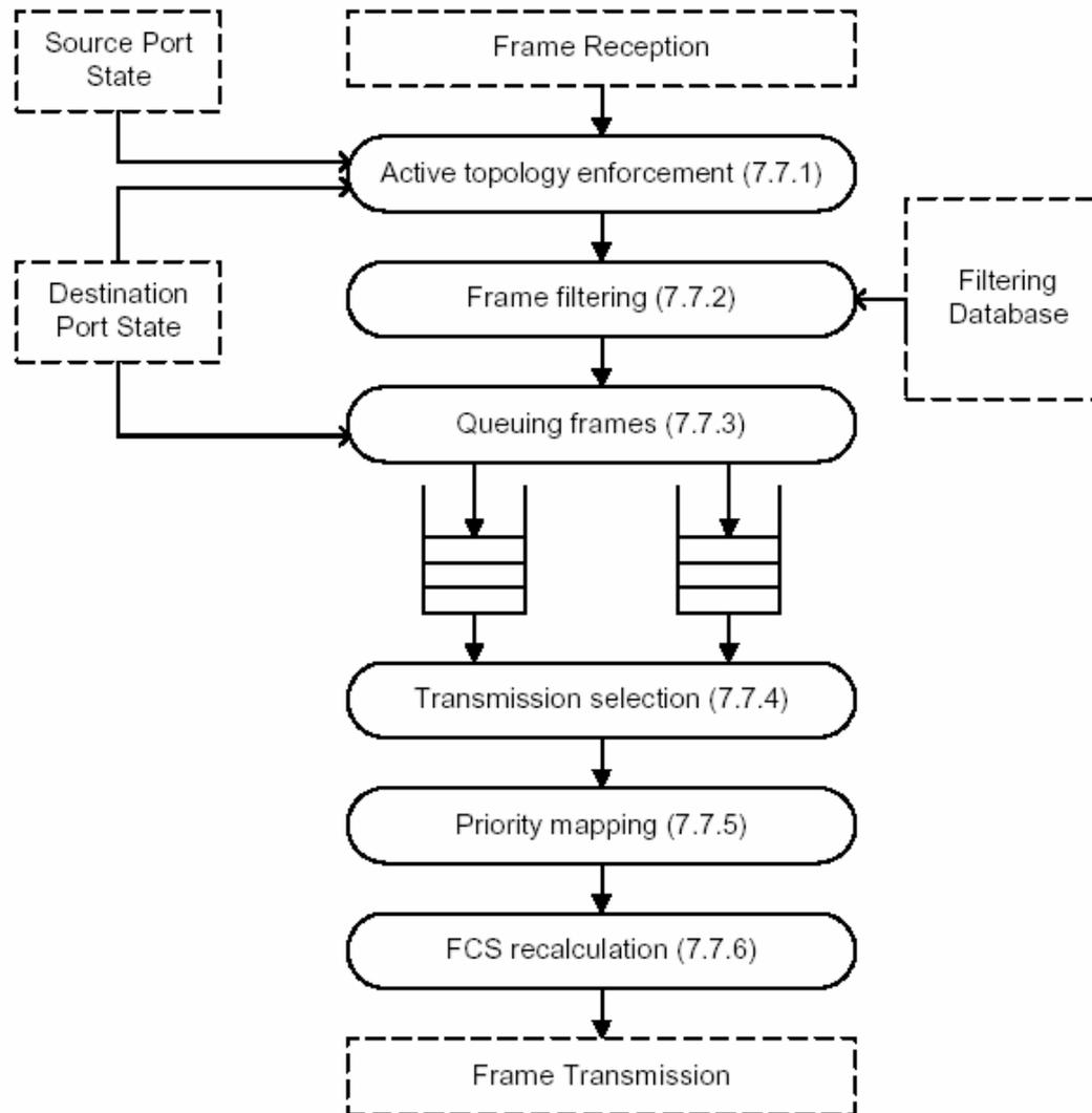
Figure 7-8—Operation of the Forwarding Process
