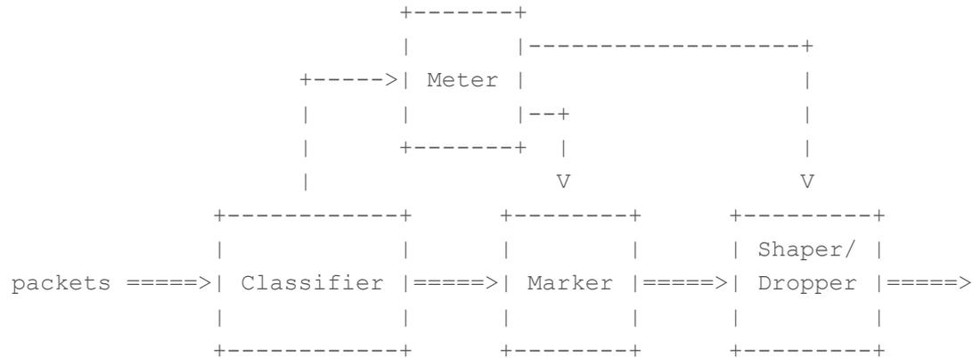
Fig. 1: Logical View of a Packet Classifier and Traffic Conditioner
