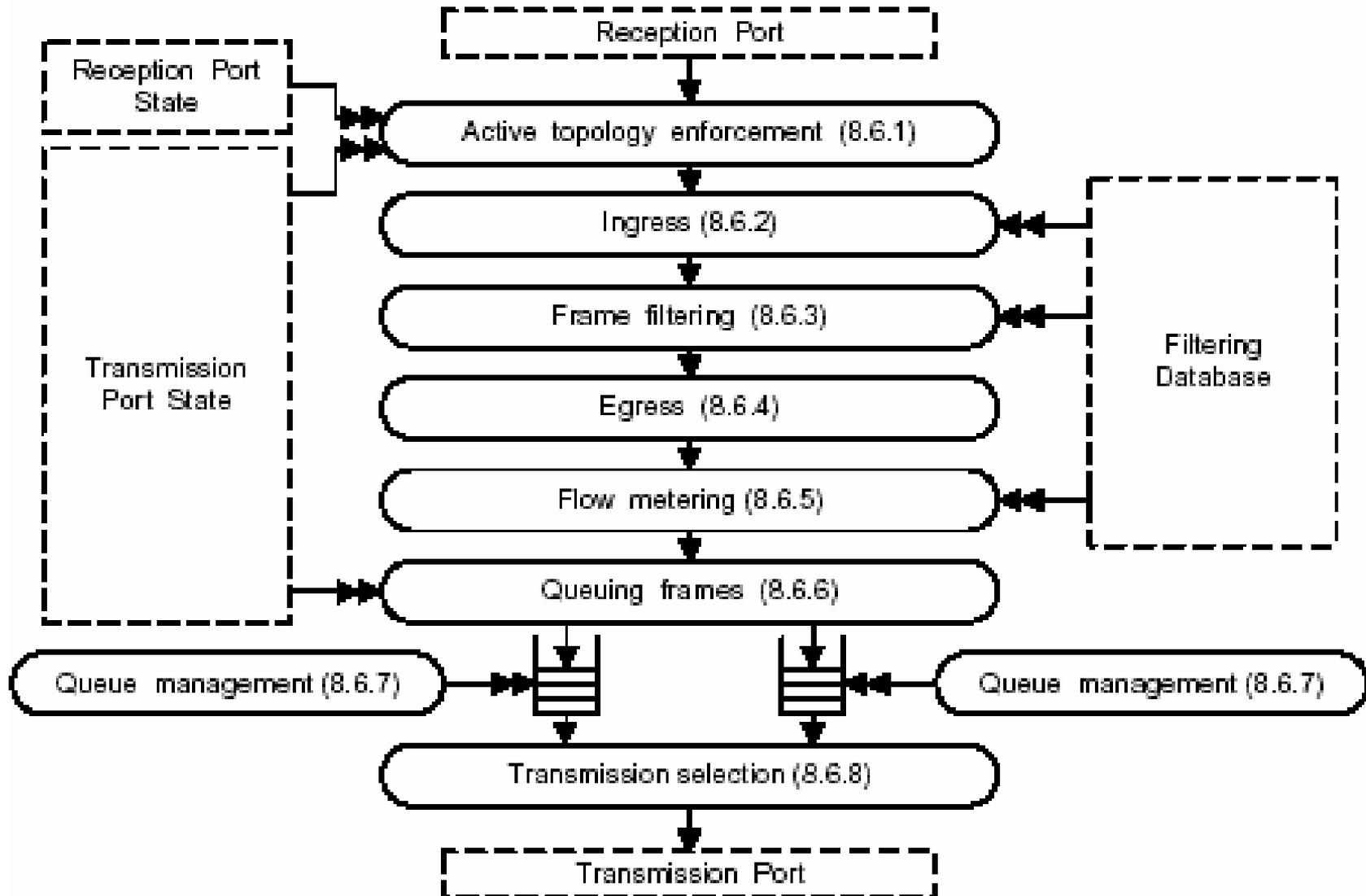
Figure 8-9—Forwarding Process functions
