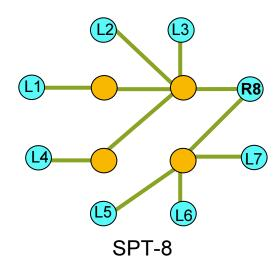
As it can be see in these figures, the path from root Rx to leave Ly on SPT-x is the same as the path from root Ry on SPT-y to leaf Lx
