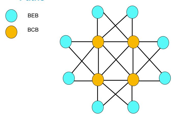
Each Bridge in PBBN runs link-state protocol (IS-IS) and thus has a full picture of the network topology
