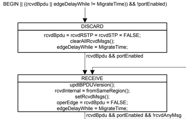
Figure 13-16—Port Receive state machine
