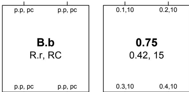
A template for and example of an STP Bridge. **B.b** is the Bridge Identifier (including the manageable priority component **B**). **R.r** and **RC** are the Root Identifier, Root Path Cost, and the Designated Bridge Identifier, for the Root Port. **p.p, pc** are the Port Identifier (with manageable priority **p**.) and the Port Path Cost for a Bridge Port.
