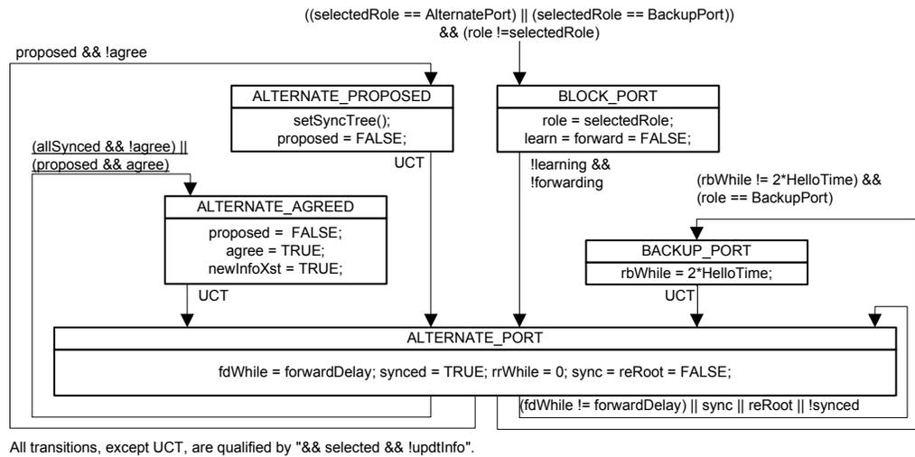
Figure 13-26—Port Role Transitions state machine—AlternatePort and BackupPort
