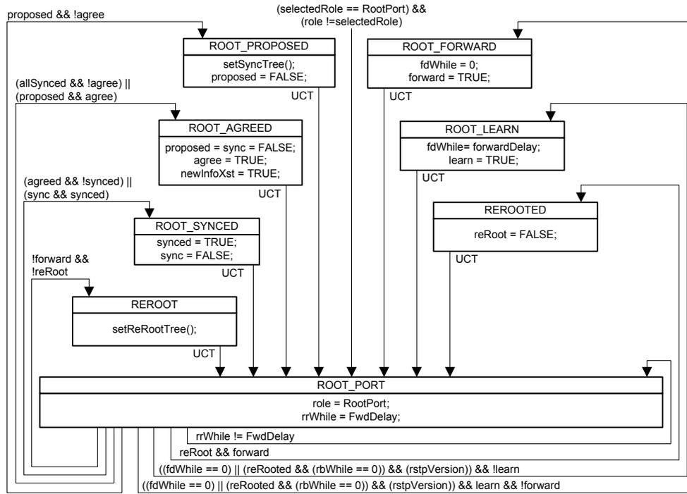
Figure 13-24—Port Role Transitions state machine—RootPort
