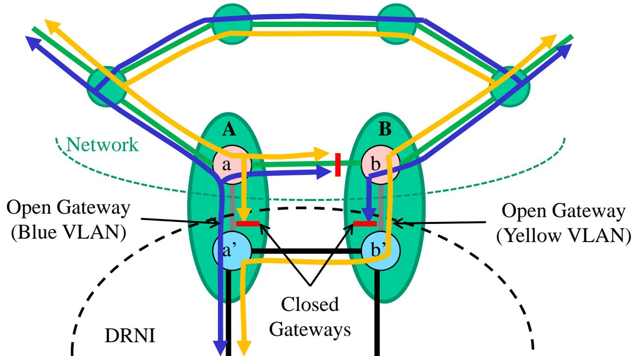
In Case D1 the network link between the DRNI nodes is either not present, is broken, or is blocked. This example shows the broadcast path for two VLANs (Blue and Yellow). The link selection for both VLANs is the same, but the gateway selection is different.
