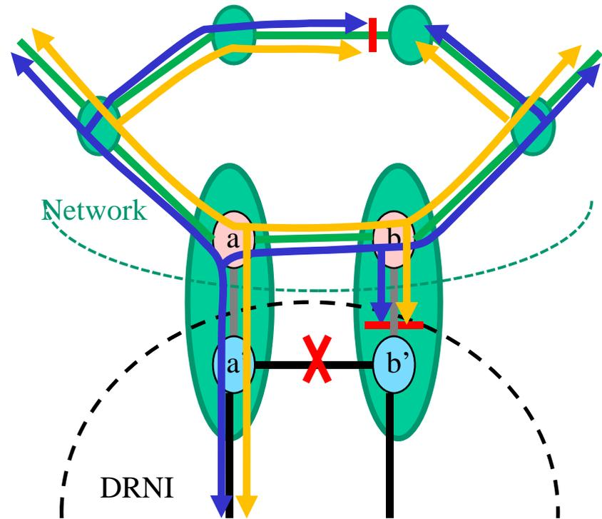
If the Intra-DAS Link failure is considered a failure in the network, then the recovery method is to change the gateway selection for any VLANs using the Intra-DAS Link. Changing the gateway reverses the direction of received DRNI frames on the path between A and B, which in this case contains the topology change to the DRNI nodes.
