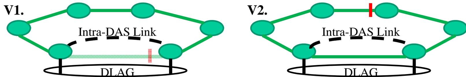
In this case the Intra-DAS Link is a virtual connection (a.k.a. tunnel) between the DRNI nodes.
