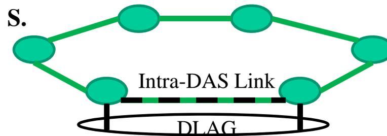
In this case there is a direct physical link between the DRNI nodes that is used both as a network link and as the Intra-DAS Link.
