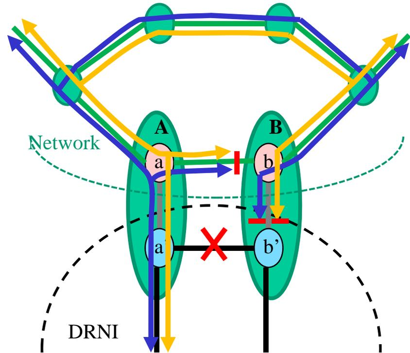
If the Intra-DAS Link failure is considered a failure in the network, then the recovery method is to change the gateway selection for any VLANs using the Intra-DAS Link. Changing the gateway reverses the direction of received DRNI frames on the path between A and B, which is a topology change in the network.
