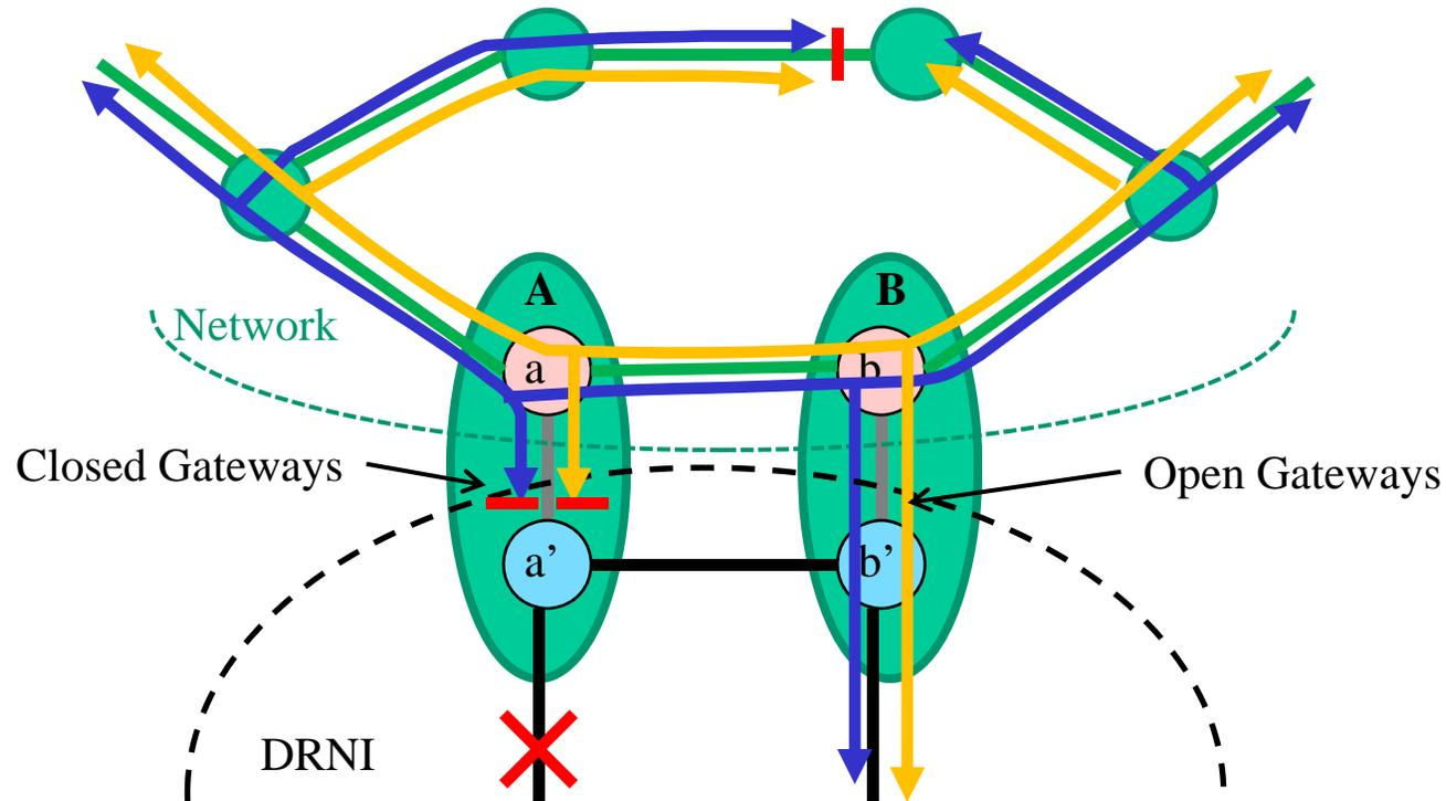
The network operator may choose to allow a change in the gateway selection as a result of the change in the link selection to make the data path more efficient. Changing the gateway reverses the direction of received DRNI frames on the path between A and B, however since the network link between A and B is in the active topology, the scope of the topology change is limited to the DRNI nodes and does not propagate to any other part of the network.
