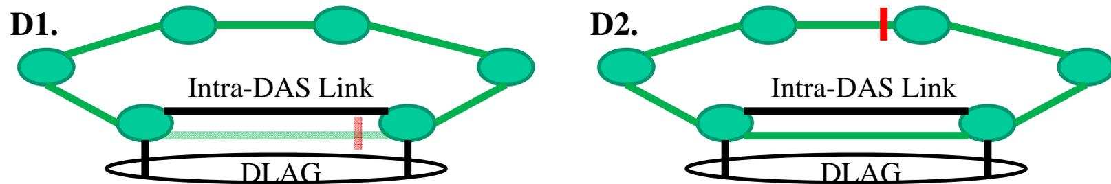
In this case the Intra-DAS Link is a direct physical link between the DRNI nodes dedicated to the Intra-DAS Link function.
