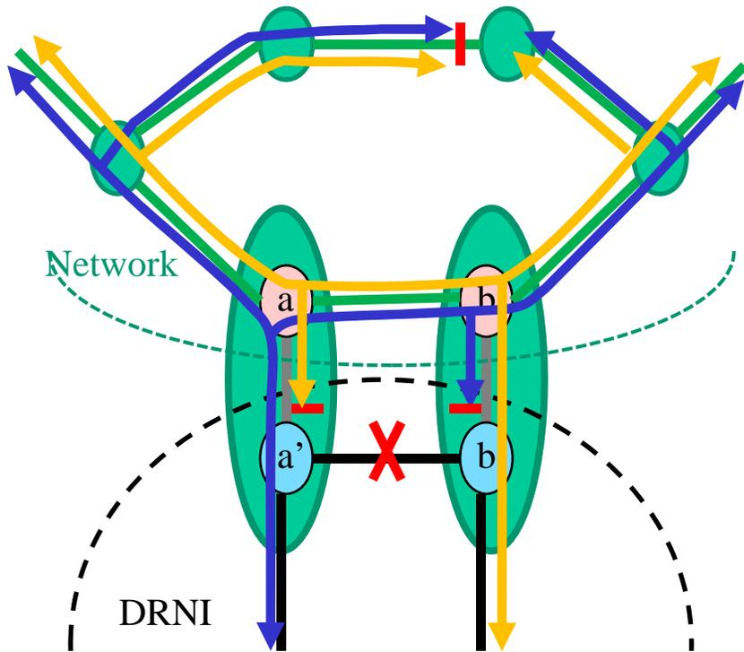
If the Intra-DAS Link failure is considered a failure in the DRNI, then the recovery method is to change the link selection for any VLANs using the Intra-DAS Link.
