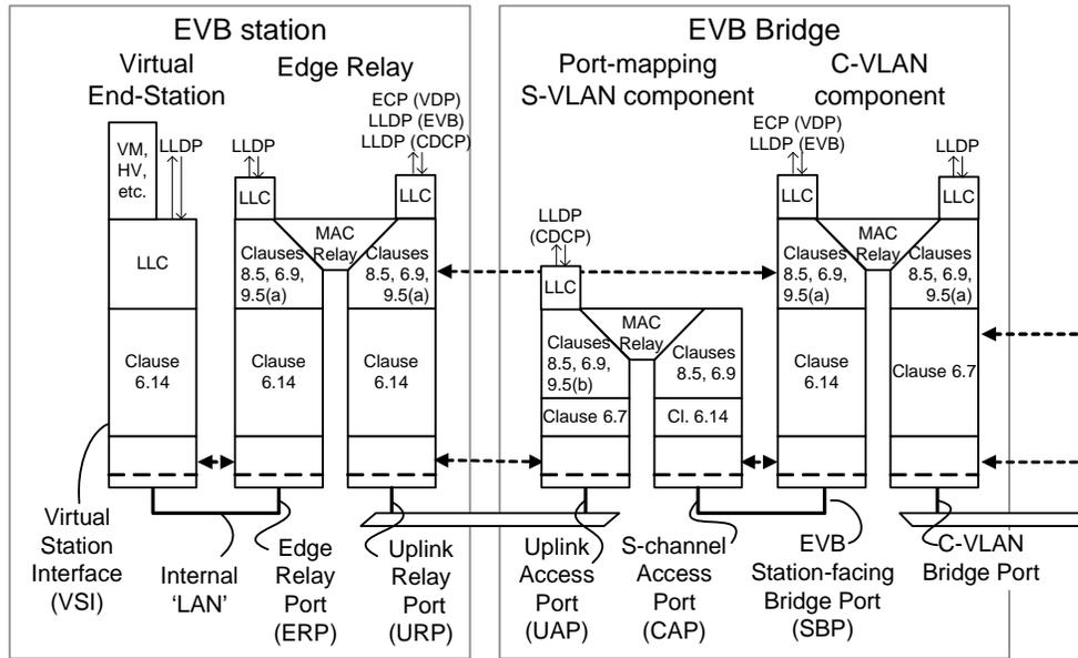
Figure 40-5—EVB architecture without S-channels including EVB Bridge S-component
