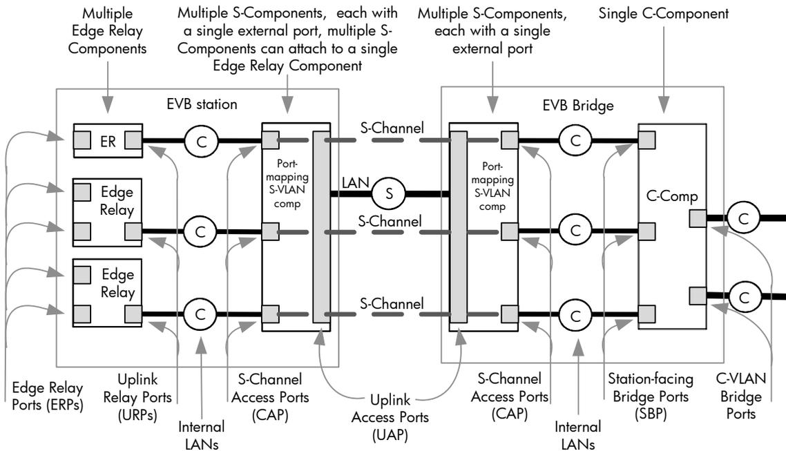
**Figure 40-4—EVB components and internal LANs with S-channels**
