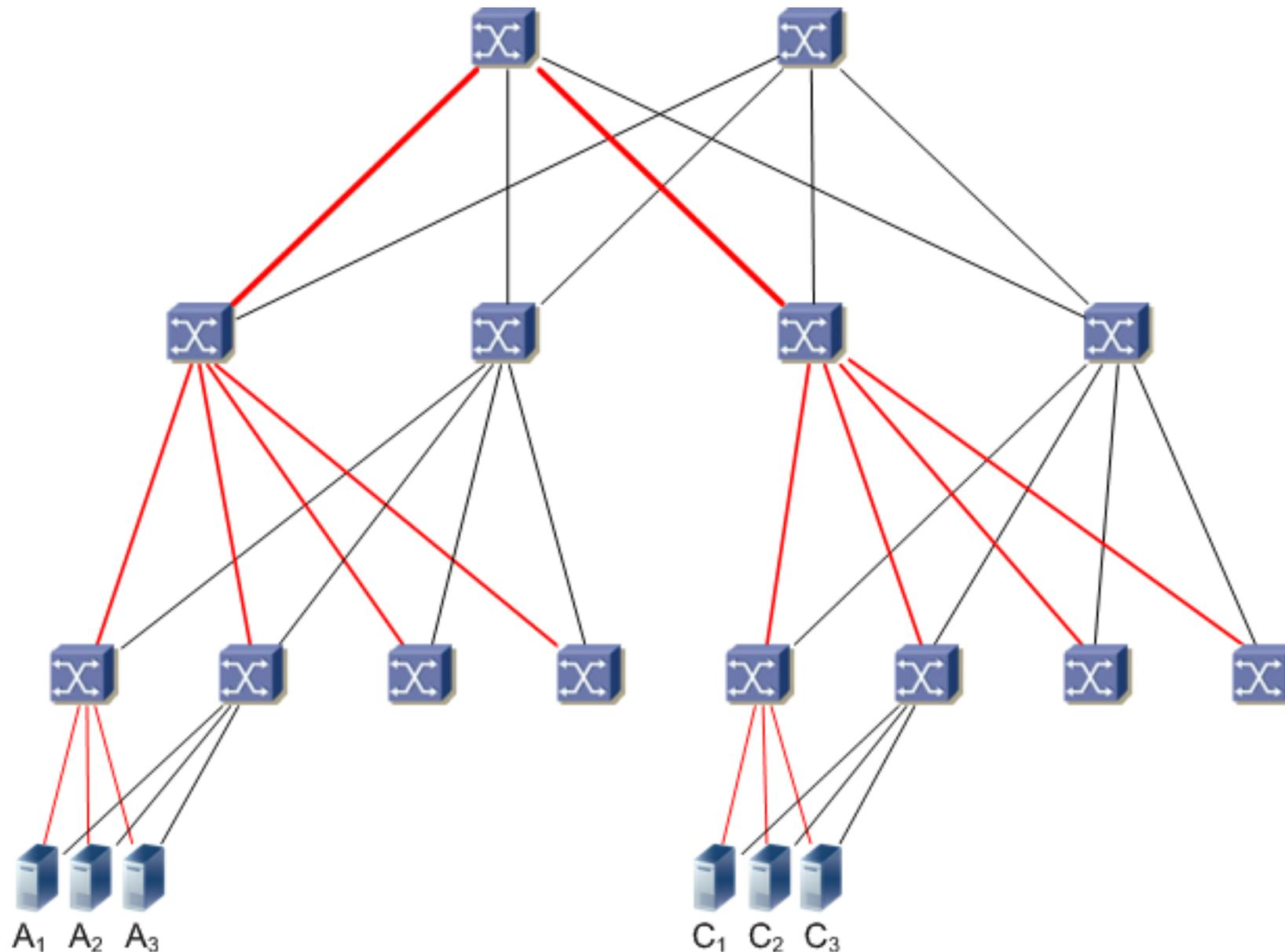
Using only one ECT-algorithm for all multicast traffic (for all service instances) can focus multicast load on a few links.
