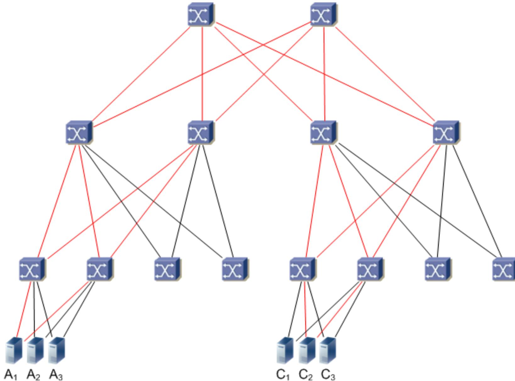
ECMP load spreading utilizes all links on equal cost paths for unicast traffic.
