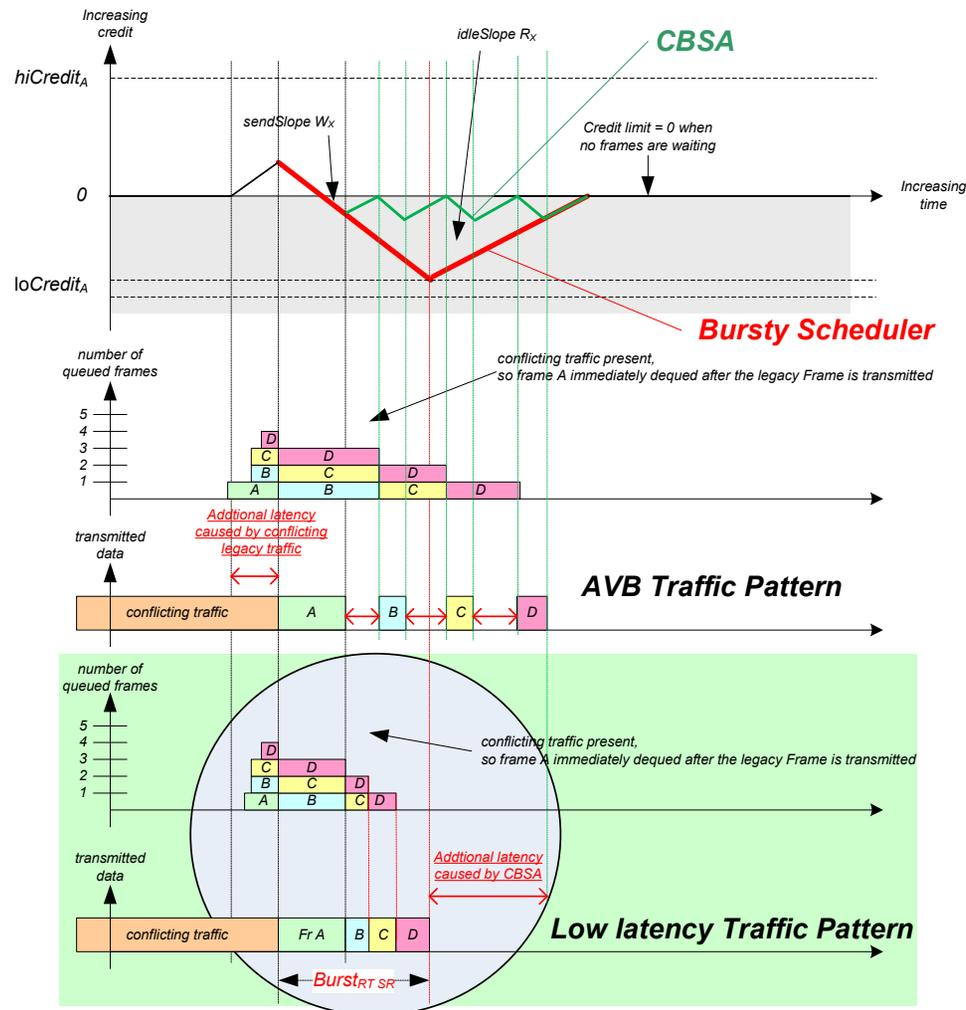
⇒ Allow bursts with max. burst size for Stream Class A' to minimize latency
