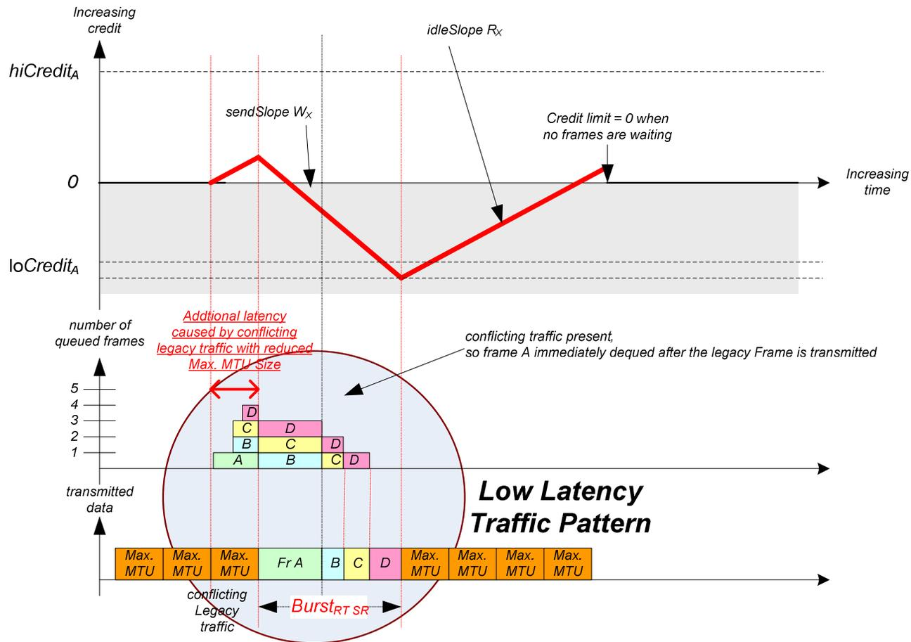
⇒ Reduce impact of large / giant interfering legacy traffic to max. MTU size but much more overhead by reduction of max. MTU Size
