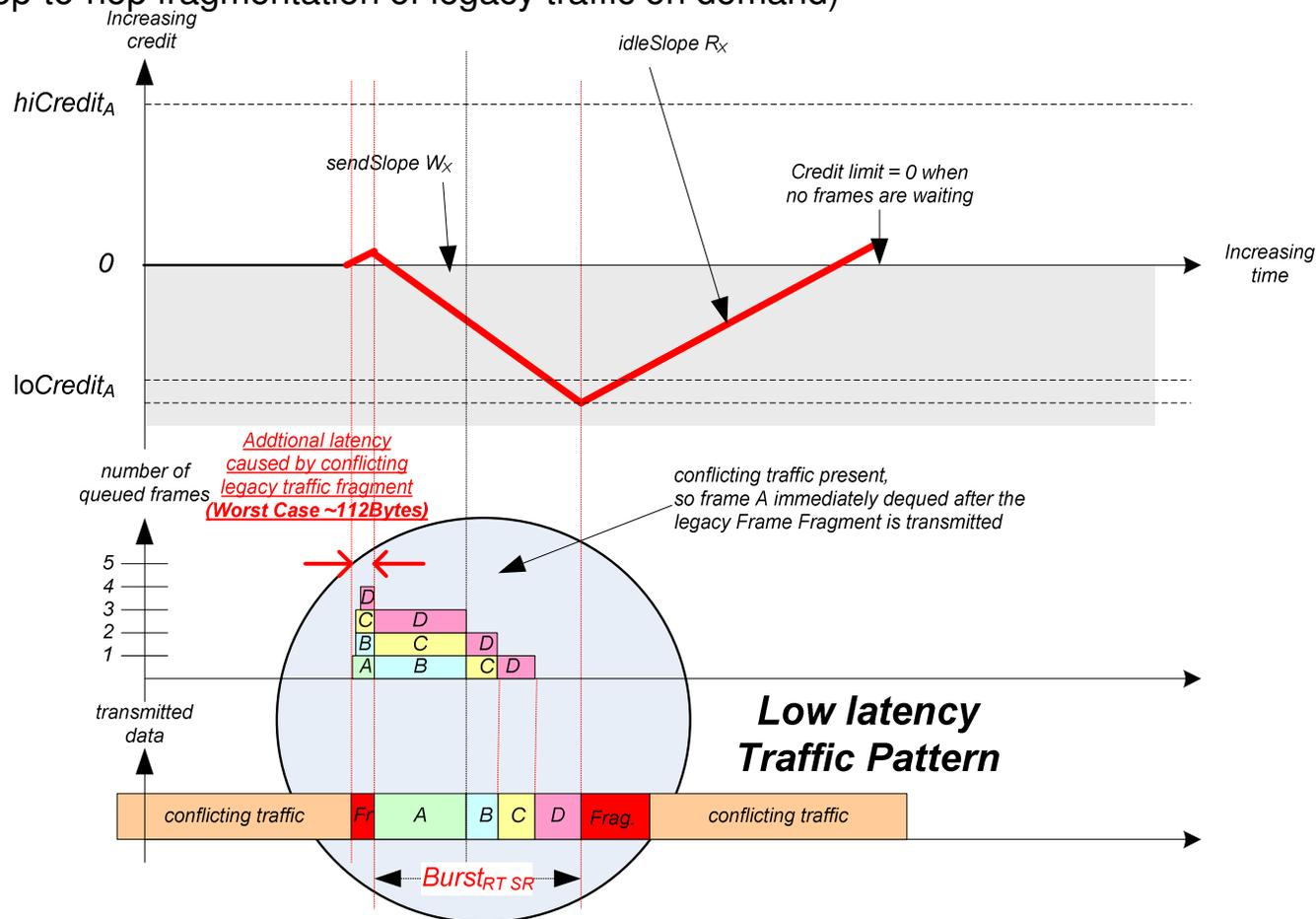
⇒ **Reduce impact on latency of large / giant interfering legacy traffic by fragmentation**
