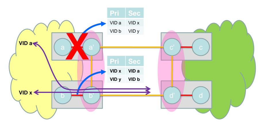
• Gateway fault causes peer gateway activation of secondary services
