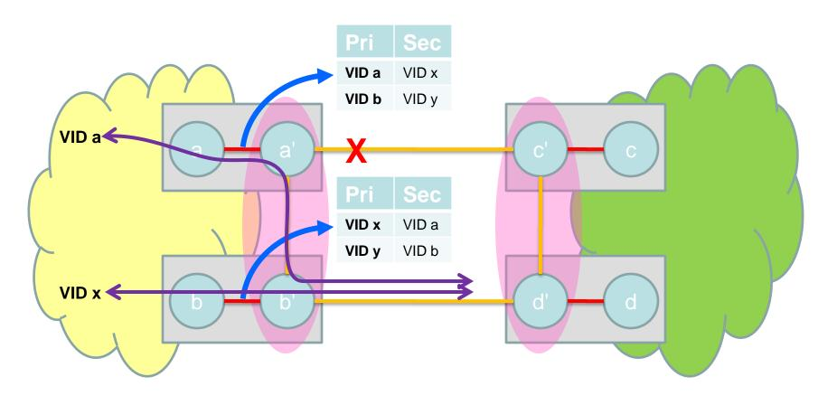
NNI fault causes D-LAG to switch
