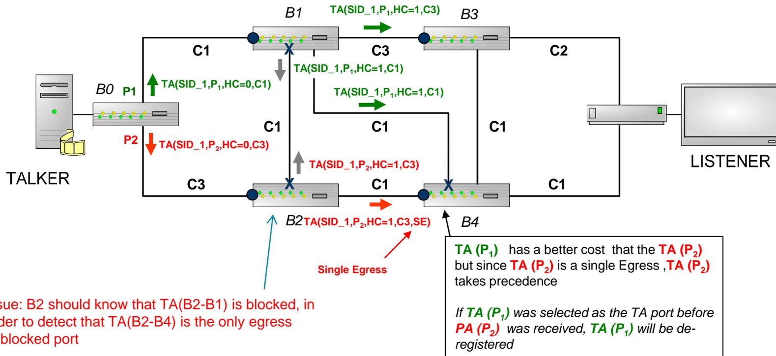
Issue: B2 should know that TA(B2-B1) is blocked, in order to detect that TA(B2-B4) is the only egress unblocked port
