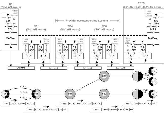
Figure 1—Interface stacks and paths for PBN tagged service interfaces
