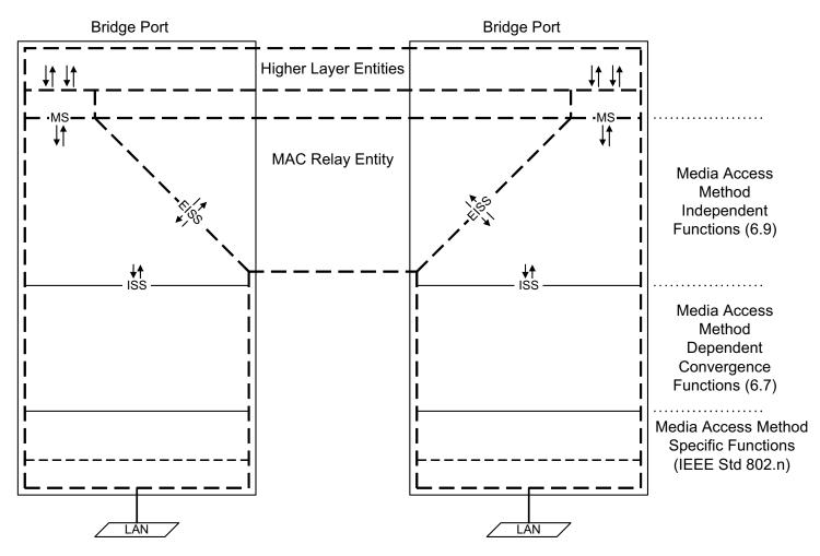
NOTE—The notation "IEEE Std 802.n" in this figure indicates that the specifications for these functions can be found in the relevant standard for the media access method concerned; for example, n would be 3 (IEEE Std 802.3) in the case of Ethernet.
