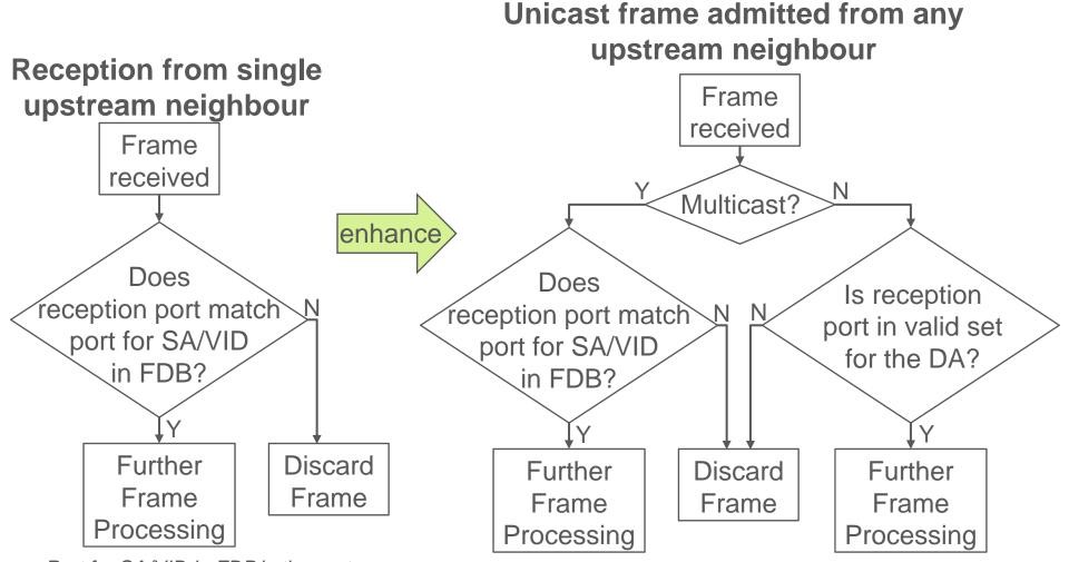
Port for SA/VID in FDB is the port providing the shortest path to SA LFA for SPBM unicast | 2013-05-15 | Page 15
