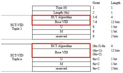
Figure 28-5—SPB Base VLAN-Identifiers sub-TLV
