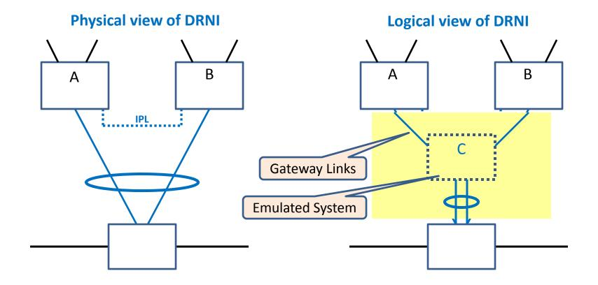
The "right" way to run RSTP across a DRNI is to have an instance of RSTP that runs in the Emulated System and exchanges BPDUs across the Gateway Links with the Portal Systems and across the LAG with the LAG Partner.
