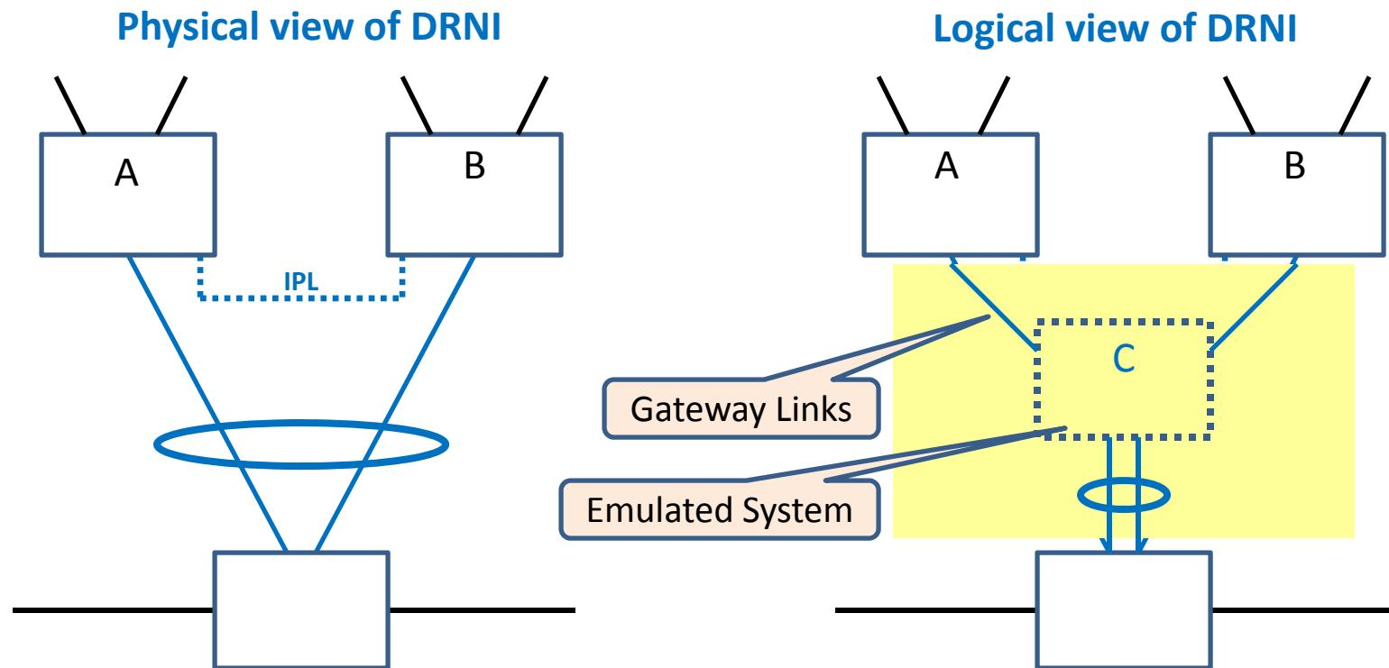
The “right” way to run RSTP across a DRNI is to have an instance of RSTP that runs in the Emulated System and exchanges BPDU<sup>s</sup> across the Gateway Links with the Portal Systems and across the LAG with the LAG Partner.
