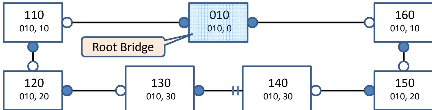
RSTP results using a link cost of 10 for each external link and 1 for the gateway links.
