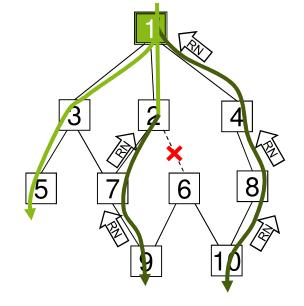
Bridges receiving RN (e.g. 9 & 10) send RN on alternate path Bridges receiving data + RN (e.g. 1 & 2) start sending on RN reception port
