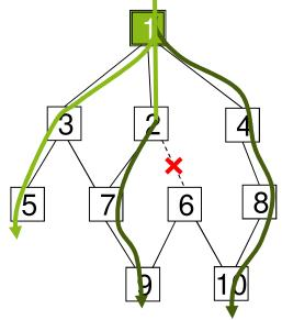
Bridges react keyed on the LSP encoding the failure
