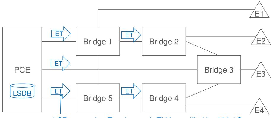
LSP conveying Topology sub-TLV specified by 802.1Qca
