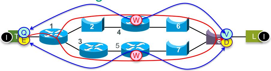
• The Interworking Functions (w) enable the TSN Pseudowire Encaps function (E) and the Sequenced TSN Decaps function (D) at the very ends of the network to be peers, just like the Sequenced TSN and IPgram pseudowire end-to-end cases.
