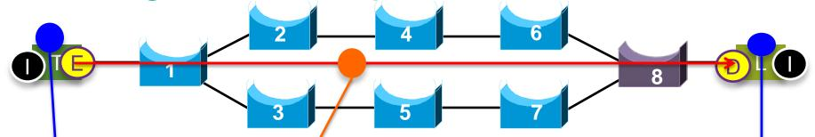
• The operator wants Talker T and Listener L to have a TSN circuit relationship , D, (734[99]) so that they can get the TSN QoS. (The bridges need the circuit ID in order to provide the TSN QoS.)
