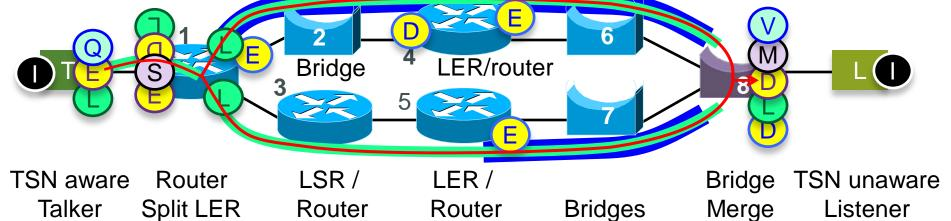
TSN Circuit Encaps/Decaps pairs are needed to convey the circuit over the various Bridged LANs. (Note the blue, instead of purple, letter and outline.)
