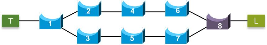
Given that introduction, let us examine the simplest case: end-to-end connectivity through a Bridged LAN. Layer 2 only: TSN tagging
