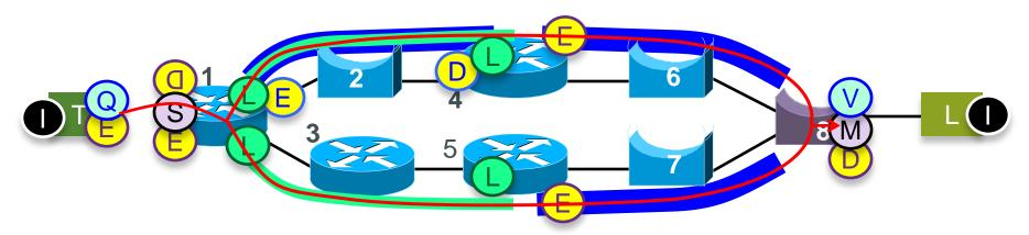
• On the right hand side, we eliminate the simple TSN encaps bused to carry the pseudowire, and replace the IPgram pseudowire encaps with the Sequenced TSN enaps that we want.
