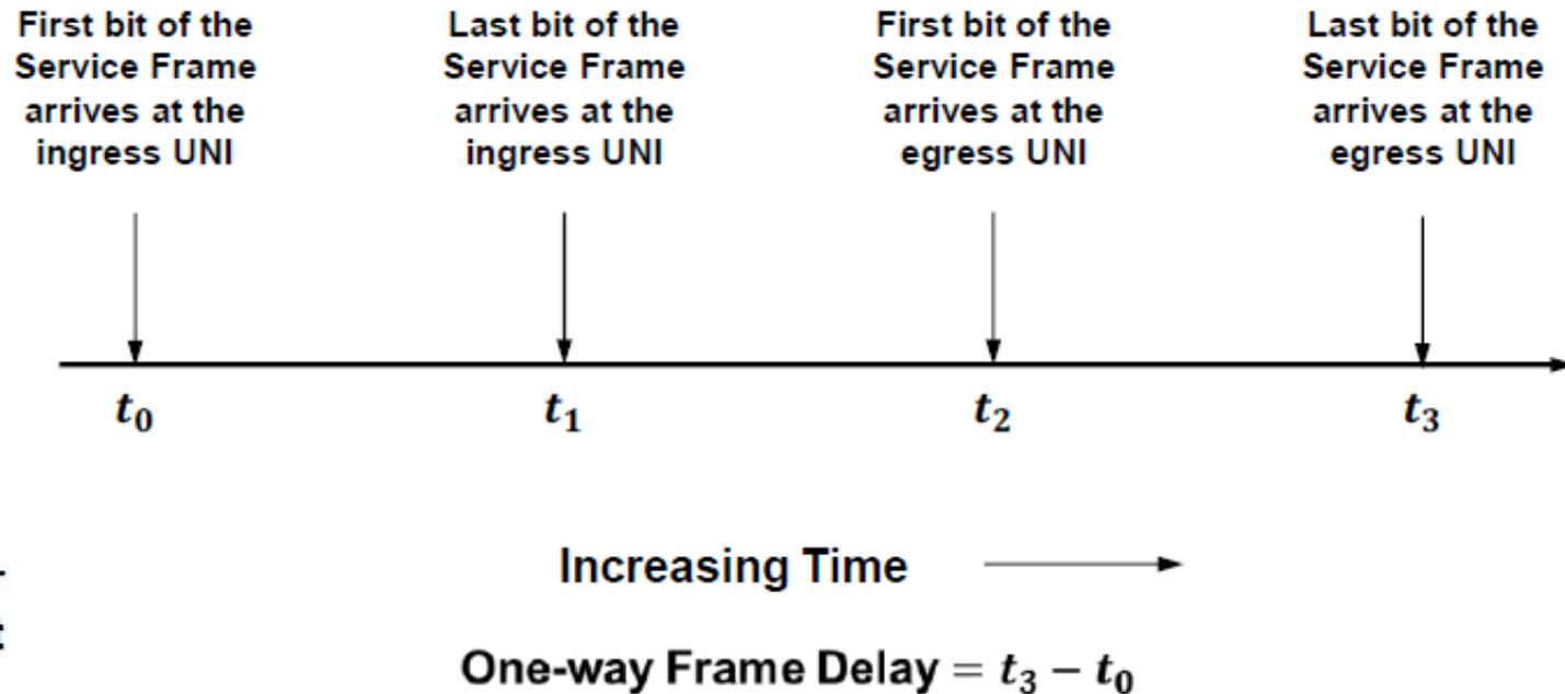
Figure 15 – One-way Frame Delay for Service Frame
