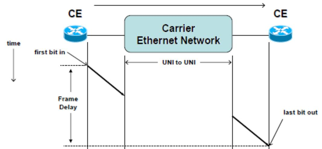
Figure 9 - Frame Delay for Service Frame
