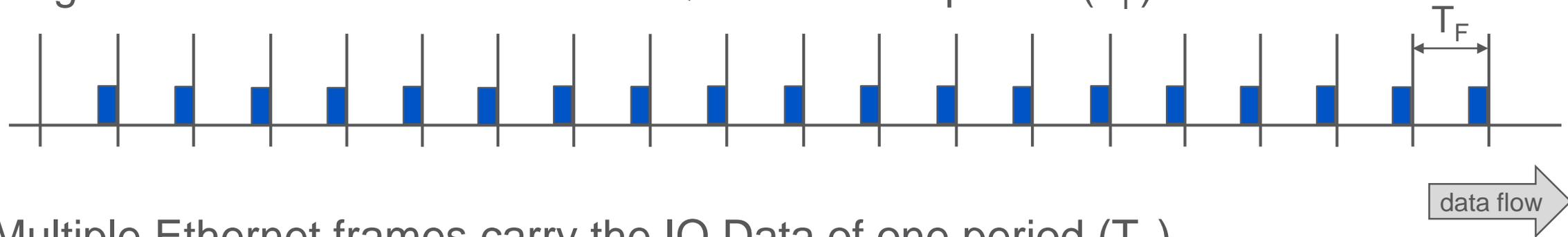
b) Multiple Ethernet frames carry the IQ Data of one period ( $T_F$ )
