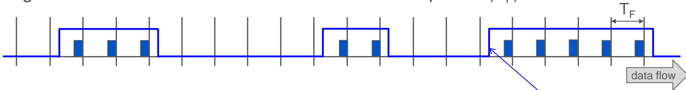
b) Multiple Ethernet frames carry the User Data of one period ( $T_F$ ) ON/OFF mask
