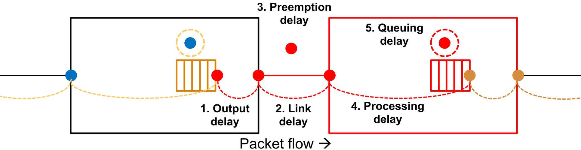
1. Output delay: Selected for transmission to PTP transmit time.
