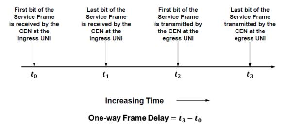
Figure 16 - One-way Frame Delay for Service Frame
